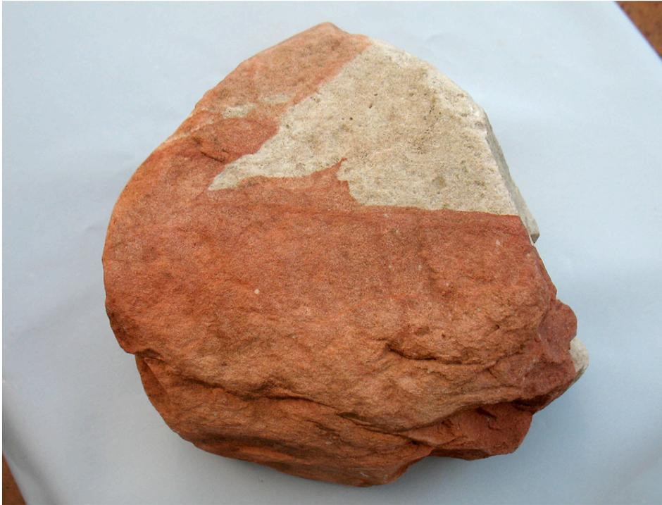
Fig. 1 Red and white Orsa-sandstone. Note the uneven contact between the two types (IMG\_2752)
