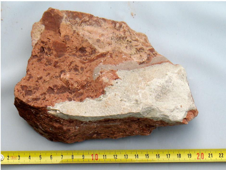
Fig. 2 Orsa sandstone from quarry at Kalmora. Note three different colours and (in the brown part) intercalated flakes of Silurian shale (IMG\_2011)
